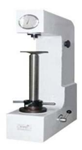
Rockwell hardness measurement of ferrous metals, non-ferrous metals and non-metallic materials.
